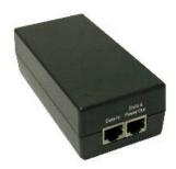
First, determine whether your system's Ethernet switch provides PoE. If so, connect one end of the supplied Ethernet cable to one of your switch's PoE-enabled ports, and the other to the RJ-45 jack on the underside of the controller.
