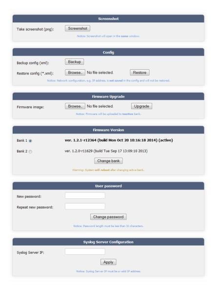
The Web GUI can be viewed with a browser on a computer on the same network as the VSet and its hybrid / Vx Engine. With HTTP Server enabled on the VSet, key the IP address of the VSet into a web browser and you will be asked to log into the VSet.
